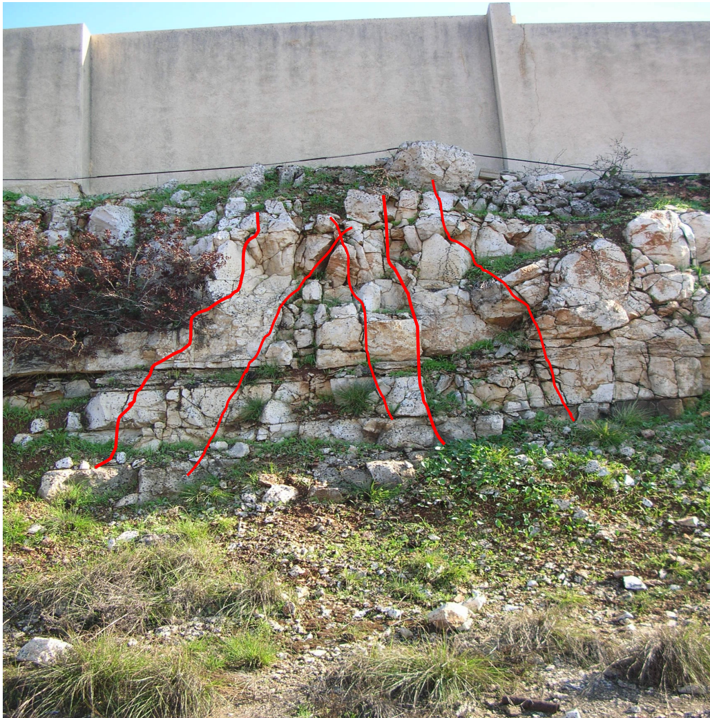
Fig. 7 : High fractured limestone beds. Notes layering in landslide attitude (“traverpoggio”), two families of joint with very narrow persistence and cavities in fracture’s plane (STOP 5)
